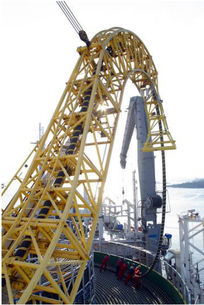
Figure 25.7. Laying a high-voltage DC link between Finland and Estonia. A pair of these cables transmit a power of 350 MW. Photo: ABB.
