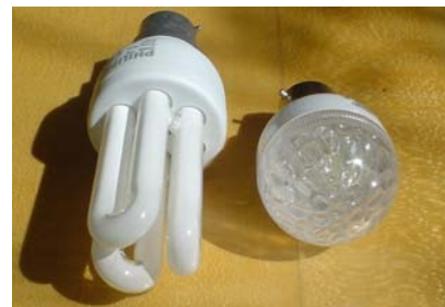
Figure 9.4. Philips 11 W alongside Omicron 1.3 W LED bulb.
