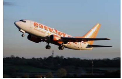
Figure C.11. Boeing 737-700: 30 kWh per 100 passenger-km. Photograph © Tom Collins.
